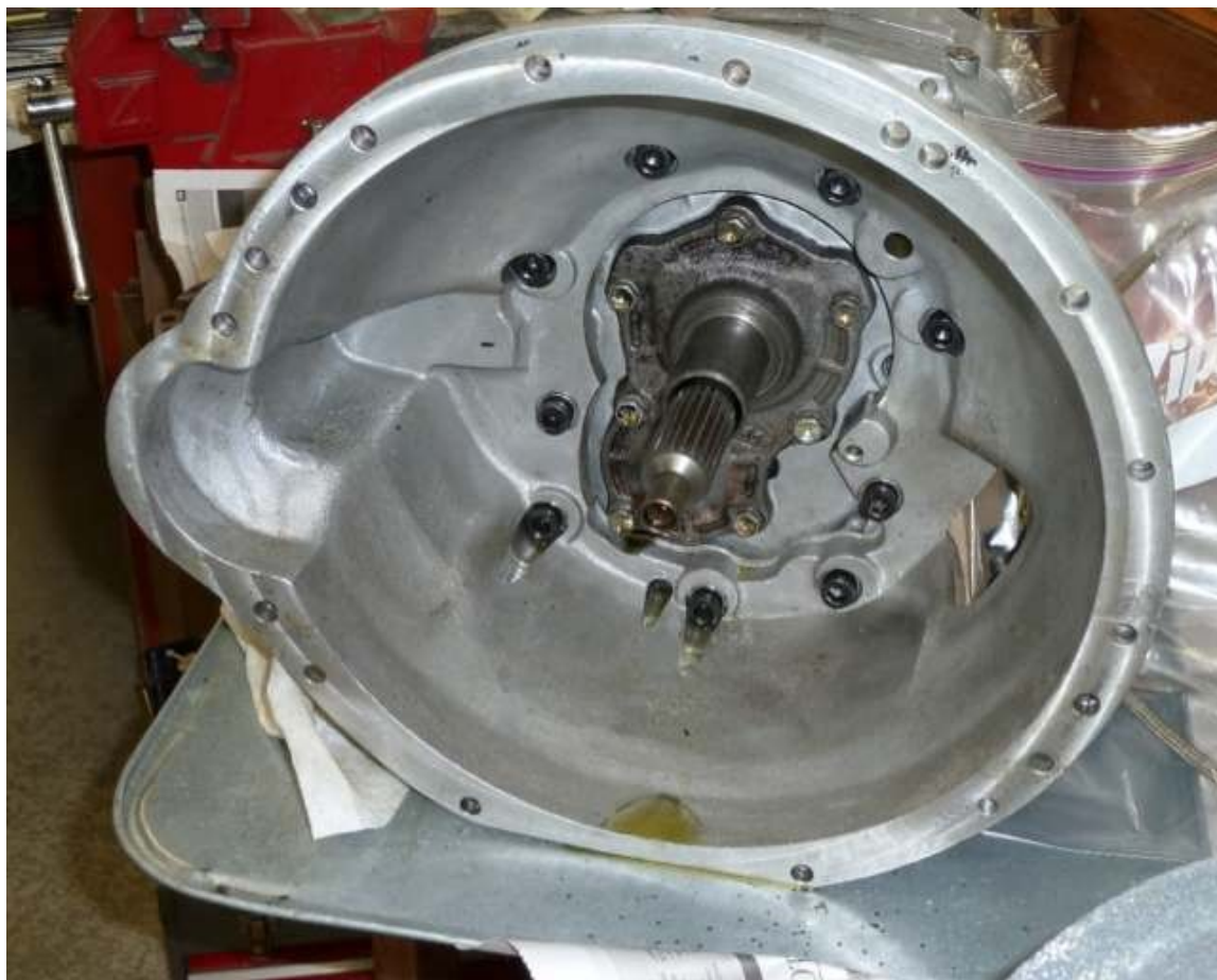
Photo 4: No wonder it leaked with no seal on the input shaft!
