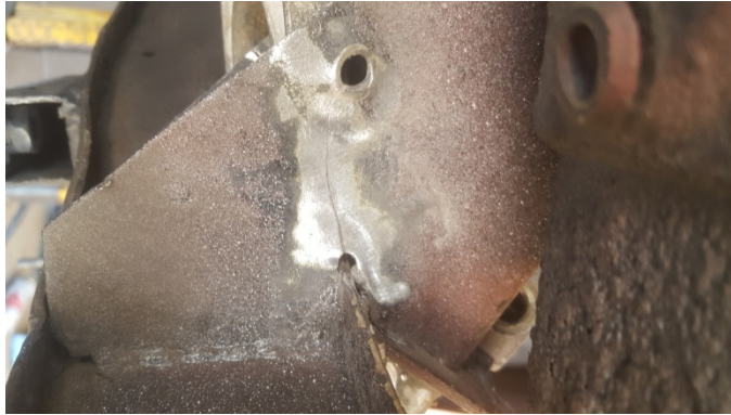
Fracture path towards drilled hole in frame.
