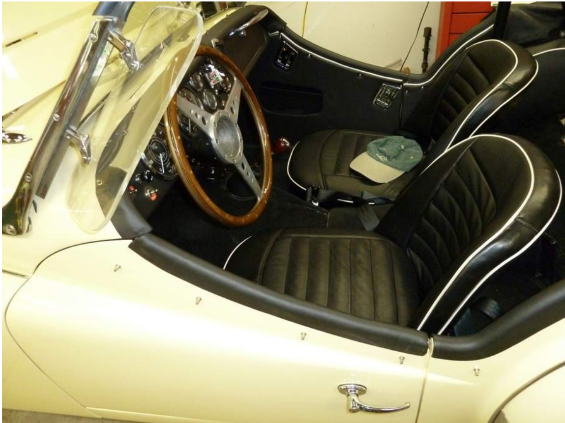
Photo 1: Modified Door Capping Installed
