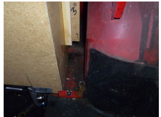
The only modification required, trimming of trunk panel attachment tab.
