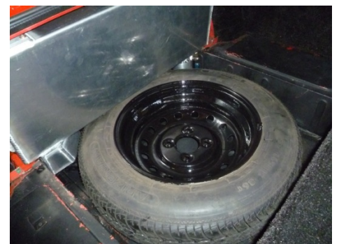
Spare tire (narrow width) just fits under the tank.
