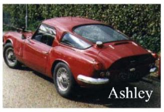
Ashley also offered a GT style top for the Spitfire similar in shape to that offered by Fibrepair, but with a more extensive backsweep to the bootlid. Though it had quarterpanel sidelights, they were high on the flanks and must have had terrrible rear vision from inside.
