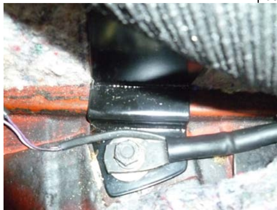
Bolted to floor underneath the seat belt anchors, very secure and stout.
