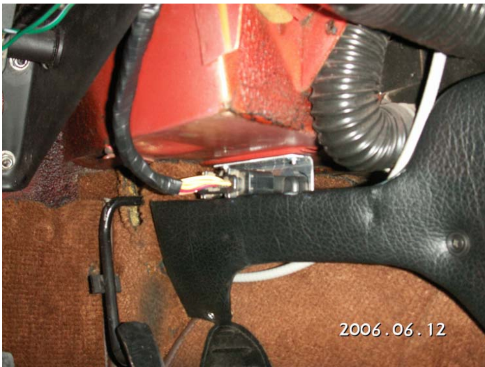
EDIS module mounted in drivers footwell
