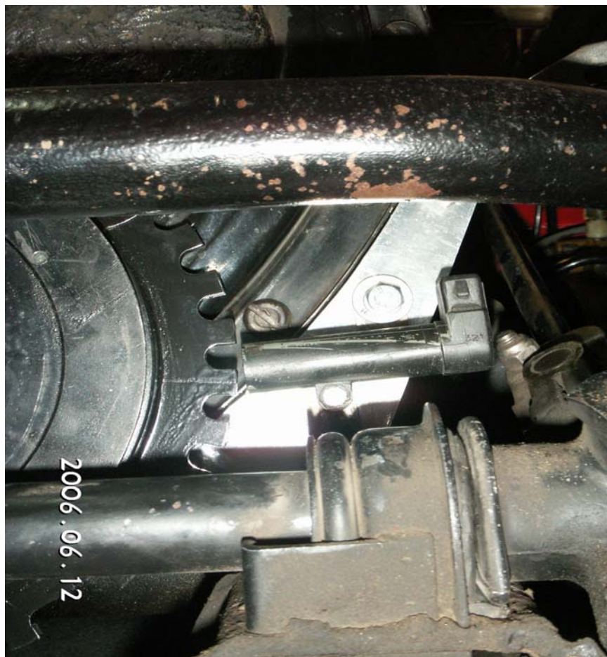
VR sensor from front of engine. It is permanently mounted about 0.060" from wheel. Mount follows contour of timing chain cover.
