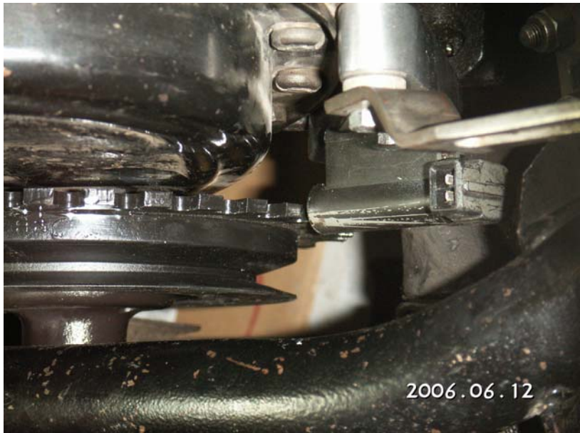
Crankshaft sensor (VR) mounted below alternator. Looking down from top of engine
