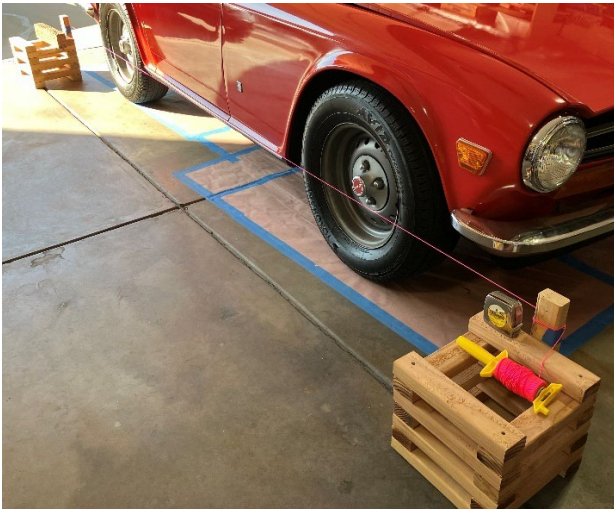
Photo 4 String set up for measurements
