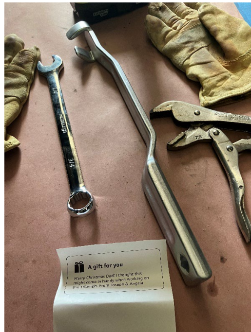
Photo: Gift wrench extender needed to free up tie rod retainer nut.
